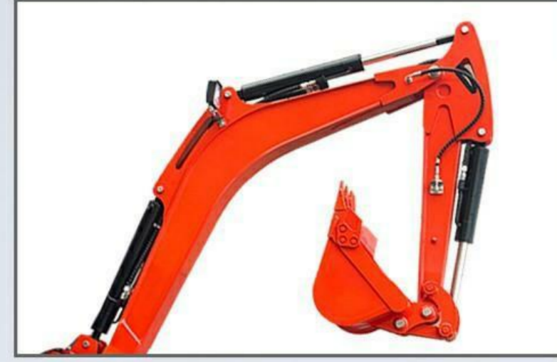
Inverted oil cylinder Hidden oil pipe.
