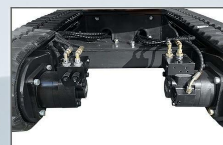
Customized oil return line traveling motor.
