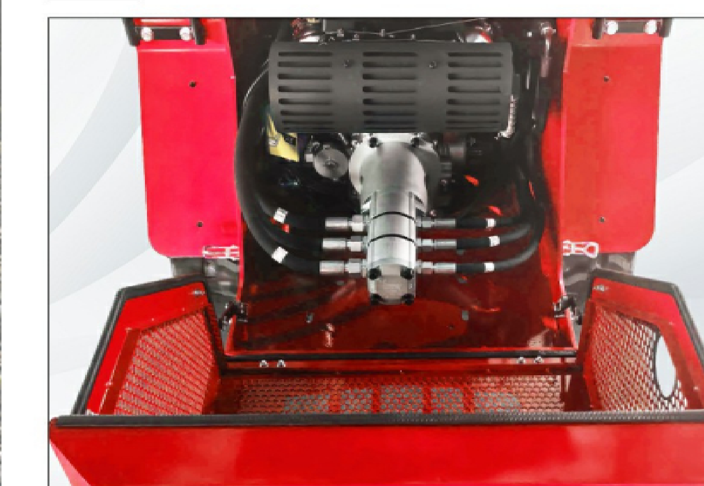
03 Rear flip cover design for easy maintenance
